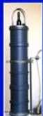
Figure 3 - Four Lotek WHS3050 76Khz Wireless Hydrophones were deployed in a thoro-fare in the Great Bay Estuary, NJ for acoustic tracking.
