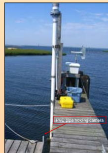
Fig. 7. Camera system in the boat basin at RUMFS.
