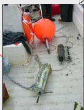
LARS setup cable tied to existing hydrophone mooring at Parkway Bridge and Grassy Channel
