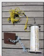
LARS setup with polypropylene rope and 15lb anchor attached at LSHC bridge
