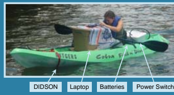
DIDSON Laptop Batteries Power Switch
