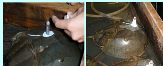
Figure 1. A Lotek CAFT11_3 ultrasonic transmitter is affixed to the carapace of a Limulus using a marine-grade, moldable epoxy and a pvc-sleeve. The protective sleeve was needed to prevent tag breakage by the horseshoe crab.
