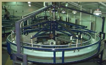
Figure 4 – Annular flume in the IMCS Seawater and Flume Facility (from http://marine.rutgers.edu/flume/annular.html )
